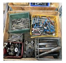
MILLING CUTTERS, DRILLING CUTTERS, TURNING TOOLS, BORING TOOLS
